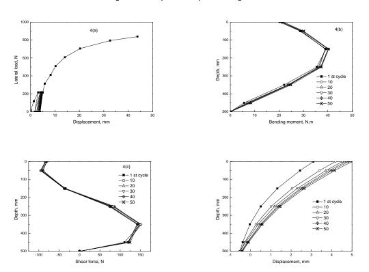
Figure 4: Response of pile during test TC1
