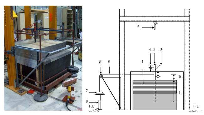
Figure 1(a): Photograph of the experiment set up Figure 1(b): Schematic diagram of the equipment 1.storage box; 2.model pile; 3.strain gauge wires; 4.LVDT; 5.steel wire; 6.pulley; 7.dead weights; 8.hydraulic jack; 9.vertical hydraulic jack
