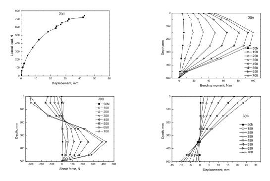
Figure 3: Response of pile during test TS1
