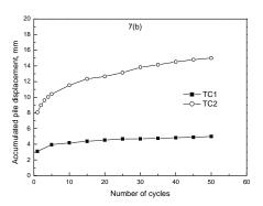
Figure 7: Critical pile response with number of cycles
