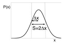
Figure 2: Squeezed states predict a Gaussian distribution for x with variance  $\Delta x = e^r$ . The measurement of a  $\Delta p$  would imply superpositions of  $|x\rangle$  that have a range (or size) S where  $S > 2/\Delta p$ . For the squeezed state,  $S > 2\Delta x$ .
