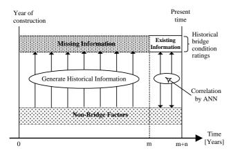
Fig. 1:Mechanism of BPM [3]
