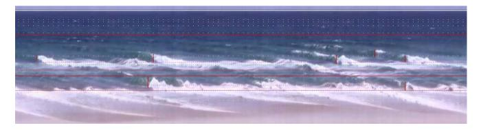
Figure 2: Section of timestack image with breakzones detected (between each solid and dotted horizontal red lines), swash zone (first horizontal dotted line in outer breakzone or green line), outer break point (second horizontal dotted line in outer breakzone or purple line) and measured breaking wave heights (vertical segments in red). The horizontal dotted white lines represent different distances while the solid white line represents the calculated horizon.
