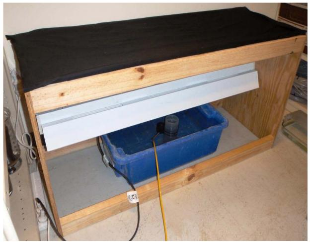
**Figure 1:** The waterproof IL1400 detector with the UVB fluorescent lamp housed inside the felt covered measurement enclosure custom built for the chemical film and monolayer UV exposure trial series.
