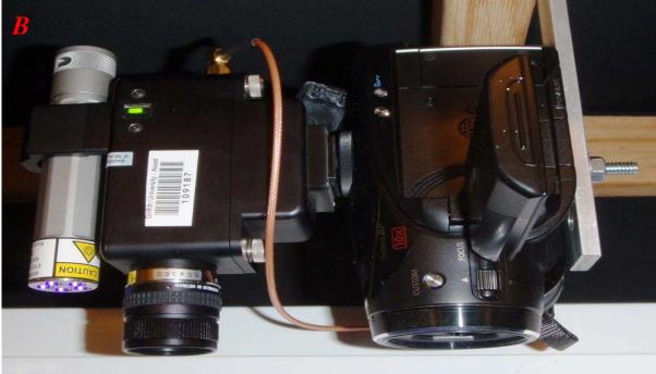
**Figure 3:** (A) The UVCorder UV camera system inserted inside the felt covered tank enclosure. (B) A close up of the UVCorder UV camera system with the 396 nm UV source tube, the CCD UV detector and the camcorder connected from left to right.
