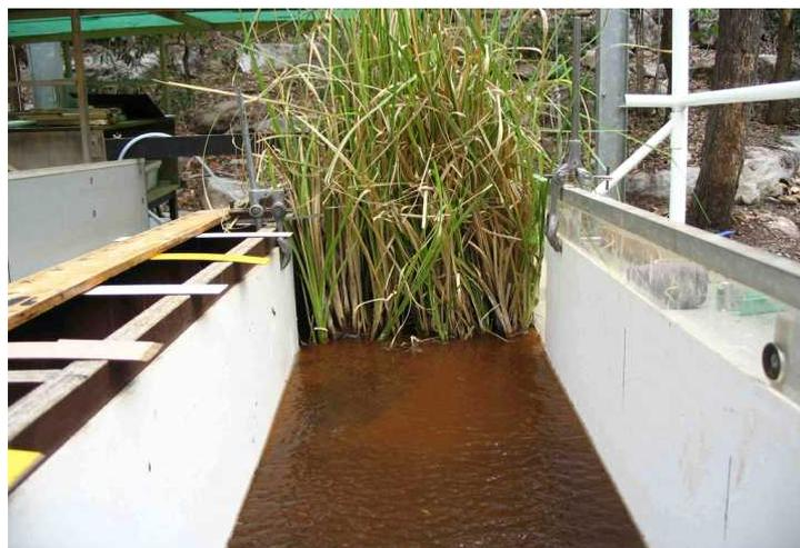
**Fig 2. Zone of backwater upstream of the Vetiver buffer strip**
