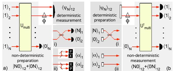
FIG. 1: Non-deterministic a) preparation & (b) measurement of NOON-states for phase super-resolution, as described in text. i) photon-counting after a 50% beamsplitter to measure  $\langle N|_1$  &  $\langle 0|_2$ . ii) coherent-state detection,  $\langle \alpha_1|$  &  $\langle \alpha_2|$ , via a 50% beamsplitter and two homodyne detectors to measure amplitude and phase. (i & (ii) are the corresponding time-reversed processes.
