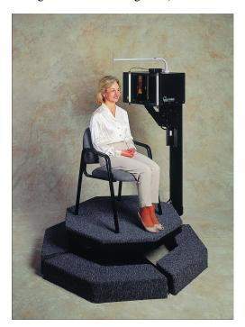
Fig. 1. The Cyberware Head & Face Colour 3D Scanner [9] and the scanning process. Two of the lamps are installed on the scanner's head to provide light sources for texture acquisition.
