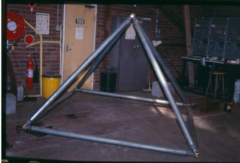
Figure 4. Pyramidal unit test of space structure
