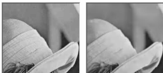
Figure 6 JPEG (L) & ShadeTree (R) at 0.5 BPP
