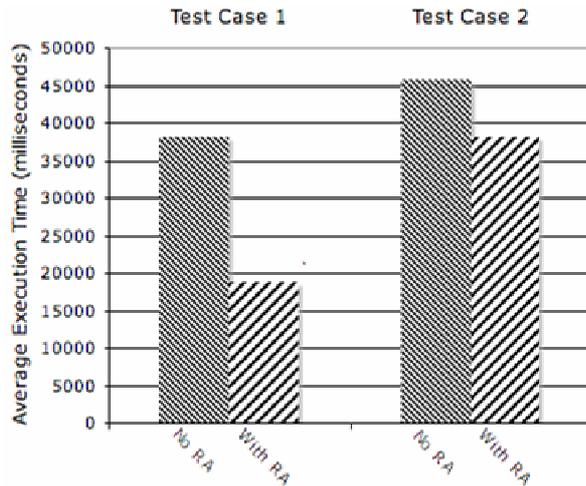
**Figure 6: Testing the grid performance with and without resource allocation (RA). Test case 1 involved nodes with significantly different performance capabilities, while test case 2 used nodes with similar capabilities.**
