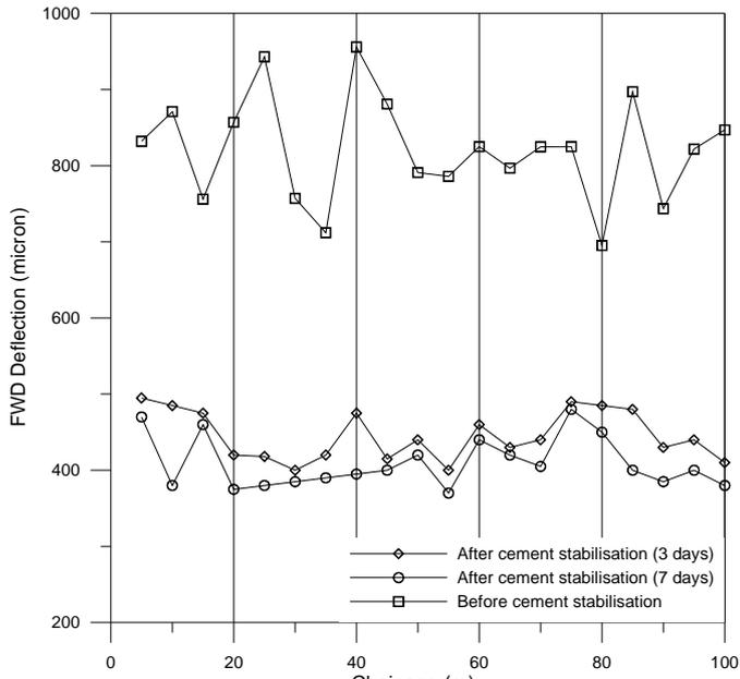
Fig. 1(a) FWD centre deflection profiles before and after cement stabilization (3 and 7 days)
