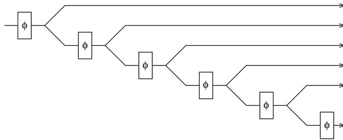
**Figure A.1.** A thought experiment intermediate between phase measurements with a NOON state and multiple passes of a single photon. The horizontal lines are photons, and the splitting indicate that the photon has been duplicated coherently.
