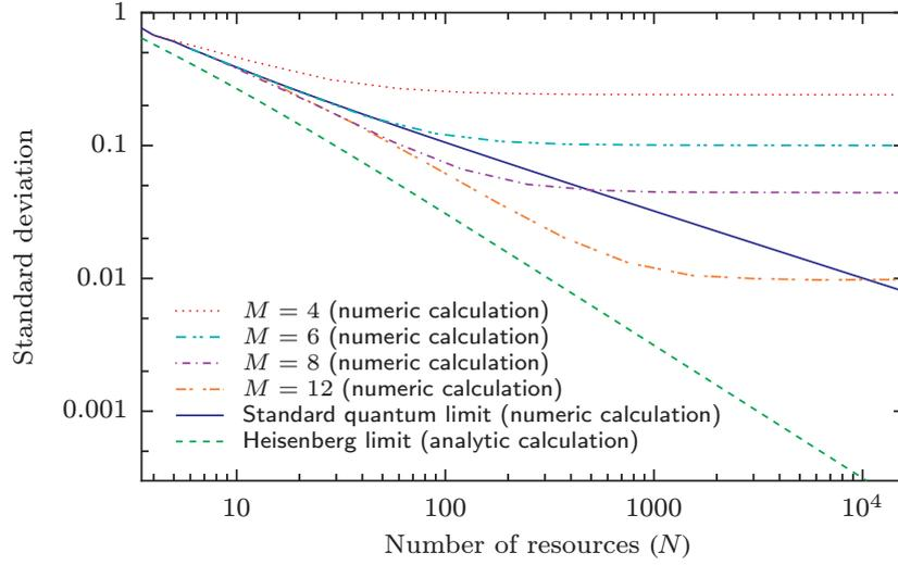
**Figure 2.** Predictions of standard deviations  $\Delta\phi_{\text{est}}$  of distributions of phase estimates under a non-adaptive scheme with fixed  $M$  and controllable phase  $\theta$  incremented by  $\pi/M$  after each measurement. Numerical predictions were based on  $2^{24}$  samples. The Heisenberg limit and the SQL are shown for comparison.
