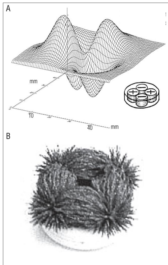
**Figure 2.** Representation of a quadripolar magnetic array. A: Field map of a quadripolar magnetic array. The magnet arrangement within the device is shown in the lower right corner (Extract from McLean et al.<sup>7</sup>). B: Pattern produced in iron filings by a quadripolar magnetic array.
