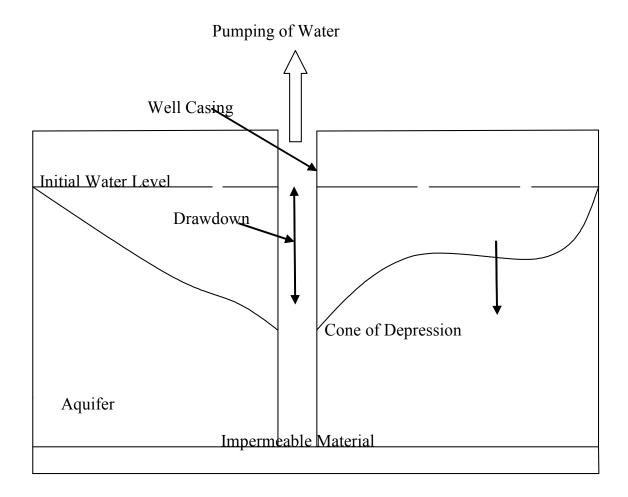
Fig. 1: A typical groundwater pumping bore.
