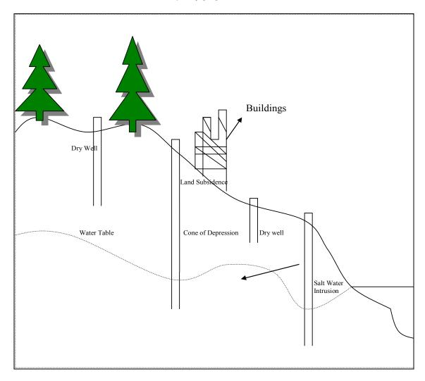
Fig. 4: Impacts of groundwater pumping
