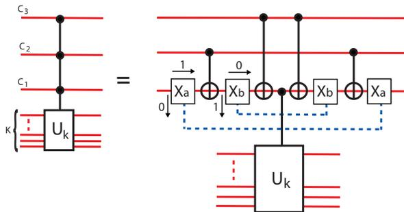
FIG. 6: Circuit for implementation of a 3-control-qubit unitary acting on  $k$  qubits,  $C^3(U_k)$ . Given the ability to perform a single instance of a  $C^1(U_k)$   $n$  additional control qubits can be added at a cost of an extra  $2n$  two-qubit gates and an additional  $n$  dimensions in  $C_1$ . The  $X_j$  perform as described in the caption of Fig. 1.
