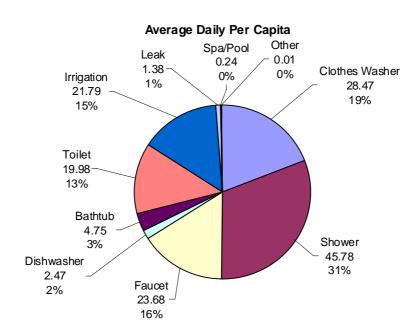
Figure 2 Gold Coast end use water consumption break down (Willis et al., 2008)
