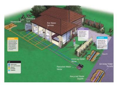
Figure 1 PCWF Master Plan – household water uses (GCW, 2004)
