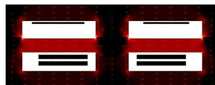
Fig.3: FEM simulation: Constructive interference of magnetic field (arrows), magnetic flux density (colour) top-up version (close to core saturation)
