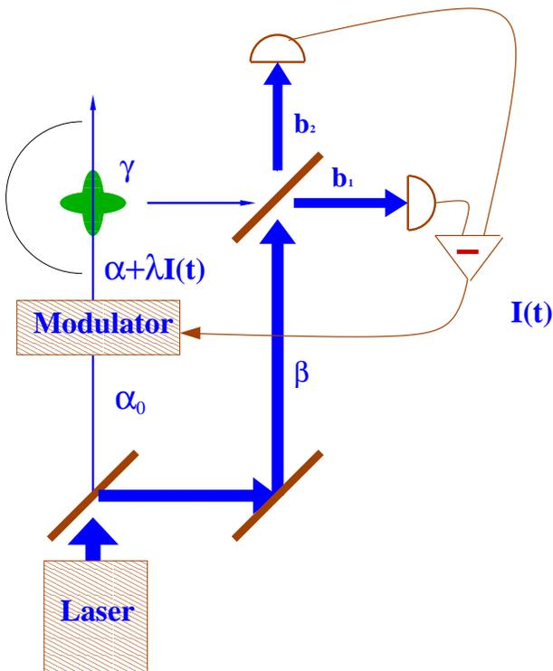
FIG. 1. Diagram of the experimental apparatus. The laser beam is split to produce both the local oscillator  $\beta$  and the field  $\alpha_0$  which is modulated using the current  $I(t)$ . The modulated beam, with amplitude proportional to  $\alpha + \lambda I(t)$ , drives an atom at the centre of the parabolic mirror. The fluorescence thus collected is subject to homodyne detection using the local oscillator, and gives rise to the homodyne photocurrent  $I(t)$ .
