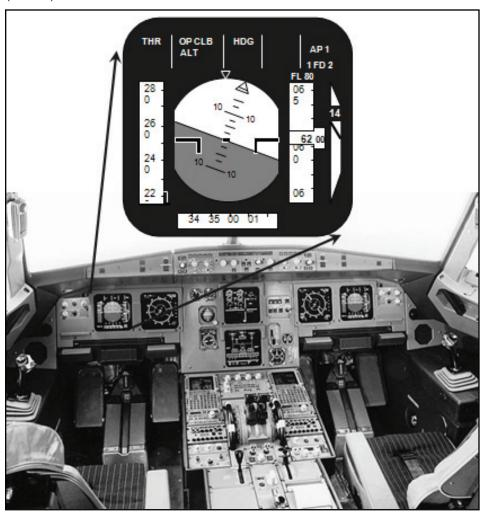
Figure 1. The Flightdeck of A320 with the FCU on the glare shield and the Primary Flight Display with the FMA above the artificial horizon. The left pilot's Primary Flight Display is magnified to show the FMA.
