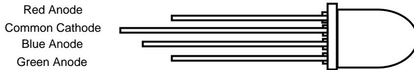
**Figure 2. Pin Diagram of RGB LED**
