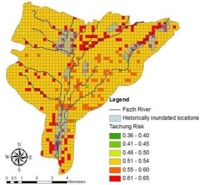
Fig. 9 Potential of inundation due to the failure of drainage systems in Fazih River with 1 kilometer buffer in Taichung City
