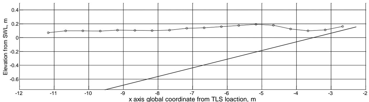
Figure 4 Maximum wave crest profile for Run 2 (dash line and circle) and beach slope (solid line)
