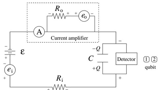
FIG. 2: A schematic of our equivalent circuit for the realistic measurement of the state of a CQD charge qubit.
